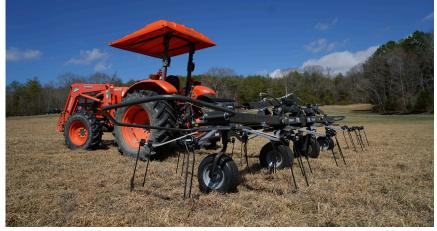
IronCraft tedders are equipped with independent rotors that can easily adapt to various ground conditions. They are available in 4 different working widths and come with a pull-type hitch. Depending on the model, the working angle can be adjusted either hydraulically or mechanically. These tedders are designed to be user-friendly and easy to transport, ensuring efficient forage distribution for quick and uniform drying.
