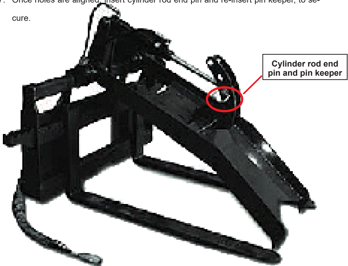
FIGURE 5.4A ADJUSTING GRAPPLE TINE HEIGHT
