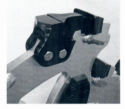
Note: Bolts have been replaced with 12 pt head bolts for an easier installation.
