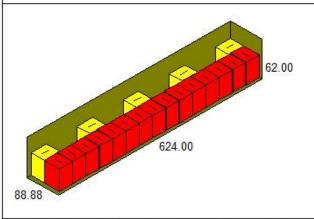
53 FT. Dry Van 636.00x98.00x110.00 Shipper UnitLoad Vehicle (OD) (Incl. Pal) Load Ln: 15.8750 in 47.625 in 624.000 in Wd: 9.1250 in 40.875 in 88.88 in Ht: 14.2500 in 62.000 in 62.00 in 40.00 lb 2080.00 lb 41600.00 lb Net: Grs: 41.50 lb 2223.00 lb 44460.00 lb Cube: 1.195 ft3 69.846 ft31989.813 ft3
