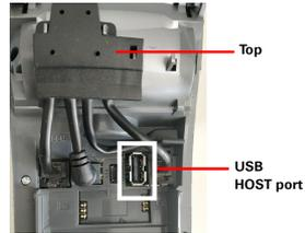
**Step 5** Plug the PIN Pad USB connector into the **USB Host** port of the terminal. **NOTE:** Ensure the PIN Pad cable is placed as outlined in Figure B.
