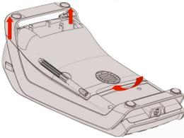
**Step 3** Remove the harness part of the terminal cable by cutting it off.
