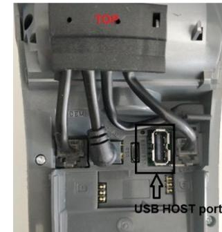
5. Plug the PIN Pad USB connector into the **USB Host** port of the terminal.
