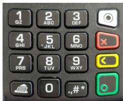
The terminal keypad is numeric only and contains 10 numeric keys (0-9), a green [Enter] key, a red [Cancel] key, a yellow [Correction] key.
