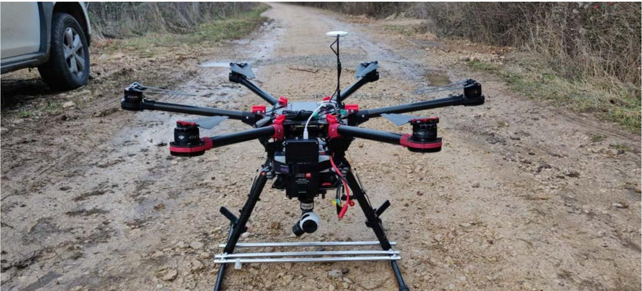
**SAF Tehnika teamed up with one of the EU's national regulatory authorities to develop a solution for precise E-band link measurement and reporting using Spectrum Compact attached to a drone.**
