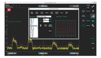
Mask mode allows using a saved spectrum curve or self-created reference line as a reference mask curve and compare it with other spectrum curves.
