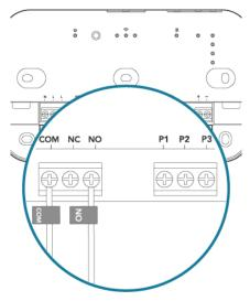
Remove the wire from terminal **NO** and insert it into the terminal labelled **COM** in addition to the wire that is already connected there. Tighten the screw. There should now be **two** wires connected to terminal **COM**.
