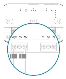
Remove the wire from terminal **NO** and insert it into one free parking terminal (**P1**, **P2** or **P3**).
