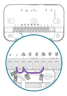
Remove the wire from terminal **HW NO** and insert it into the terminal labelled **HW COM** in addition to the purple bridge wire that is already connected there. Tighten the screw. There should now be **two** wires connected to terminal **HW COM**. Make sure that all wires are firmly connected.
