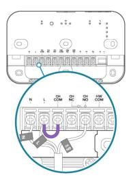
Remove the wire from terminal **CH NO** and insert it into one free parking terminals (**P1** or **P2**).
