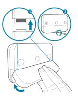
2. Put the front cover on the Wireless Receiver X.
