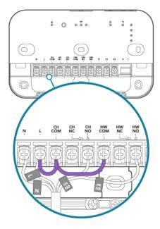
Remove the wire from terminal **HW NO** and insert it into one free parking terminals (**P1** or **P2**).
