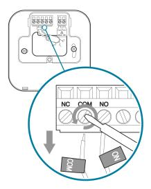
Insert the cable labelled **COM** into the screw terminal named **NO**. Tighten the screw. There should now be **two** cables connected to screw terminal **NO**. Leave the other wires untouched.
