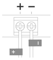
Insert the cable labelled + into the screw terminal named - . Tighten the screw. There should now be **two** cables connected to the screw terminal - . Leave the other wires untouched.
