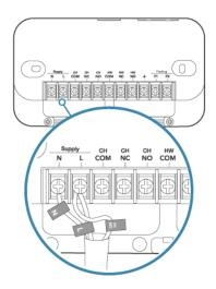
Heating always OFF - Potential Free wiring
