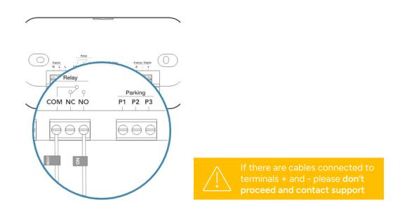
Remove the wire from terminal **NO** and insert it into the terminal labelled **COM** in addition to the wire that is already connected there. Tighten the screw. There should now be **two** wires connected to terminal **COM**.
