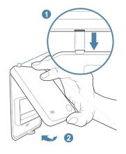
3. Push the lower part of the front cover into place. The locking mechanism produces a "click" when pushed into place. For Smart Thermostats without the automatic locking mechanism, please tighten the small screw at the bottom.
