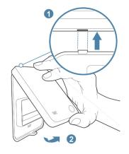
3. Loosen the security screw and unmount the terminal cover as shown in the image.
