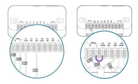
Remove the wire from terminal CH NO and insert it into one free parking terminals (P1 or P2).
