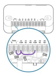
Remove the wire from terminal **HW NO** and insert it into the terminal labelled **HW COM** in addition to the purple bridge wire that is already connected there. Tighten the screw. There should now be **two** wires connected to terminal **HW COM**. Make sure that all wires are firmly connected.
