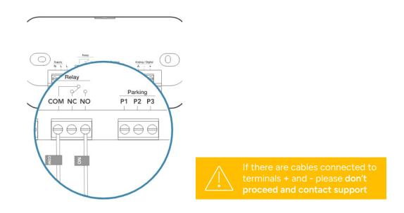
Remove the wire from terminal **NO** and insert it into one free parking terminal **(P1, P2 or P3)**.
