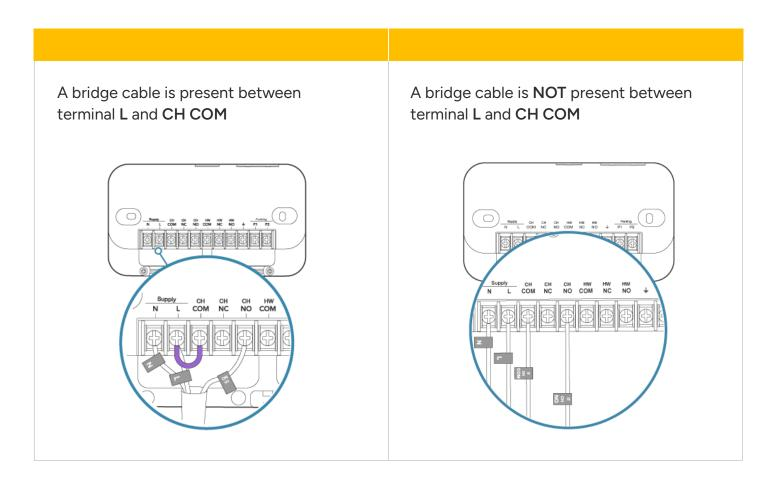
Heating always OFF - Switched live wiring
