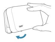
2. Tighten the small screw on the bottom edge of the tado° Wireless Receiver to firmly close it.
