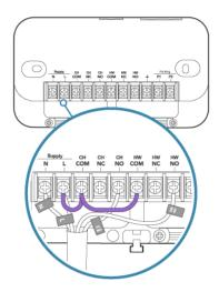
Remove the wire from terminal HW NO and insert it into one free parking terminals (P1 or P2).
