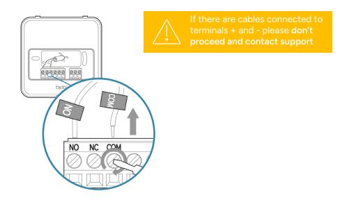
Insert the cable labelled **COM** into the screw terminal named **NO**. Tighten the screw. There should now be **two** cables connected to screw terminal **NO**. Leave the other wires untouched.
