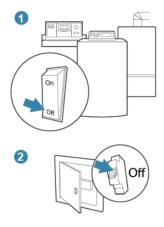
If your tado° Extension Kit is connected to a power socket, make sure that you unplug it before moving on to the next step.
