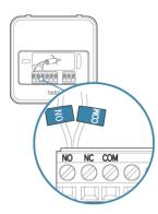
Please note that the thermostat is already bypassed if the COM and NO cables are connected by a Wago connector or are placed together in the same terminal:
