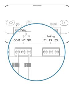
Remove the wire from terminal **NO** and insert it into one free parking terminal (**P1**, **P2** or **P3**).
