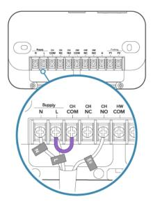
Remove the wire from terminal **CH NO** and insert it into the terminal labelled **L** in addition to the L wire that is already connected there. However, please **remove the purple bridge wire** to allow a better fit for the additional cable. Make sure to keep the bridge safe. Tighten the screw. There should now be **two** wires connected to terminal **L**.
