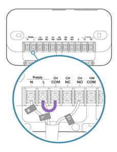
Remove the wire from terminal **CH NO** and insert it into one free parking terminals (**P1** or **P2**).
