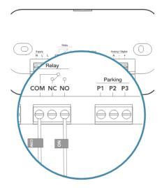
Remove the wire from terminal **NO** and insert it into the terminal labelled **COM** in addition to the wire that is already connected there. Tighten the screw. There should now be **two** wires connected to terminal **COM**.
