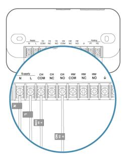
Remove the wire from terminal **CH NO** and insert it into the terminal labelled **CH COM** in addition to the wire that is already connected there. Tighten the screw. There should now be **two** wires connected to terminal **CH COM**.
