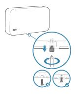
2. Remove the front cover to get access to the connection terminals.
