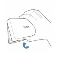
Move the Extension Kit upwards to clear it from the hinges. Leave the Extension Kit untouched and do not change the jumper position.
