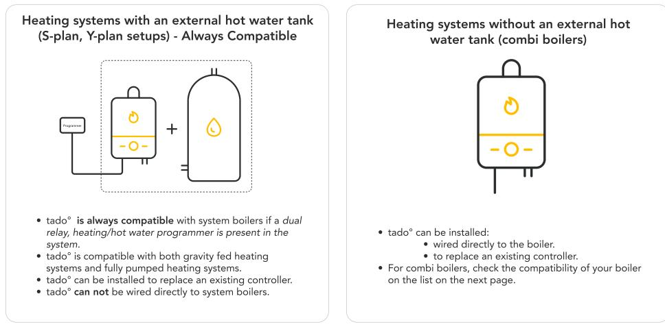
**Note:** If you need to control a dual relay system for central heating and hot water, you will require the Wireless Smart Thermostat Starter Kit with Hot Water Control. tado° X and V3+ are both compatible with heating systems with an external hot water tank.
