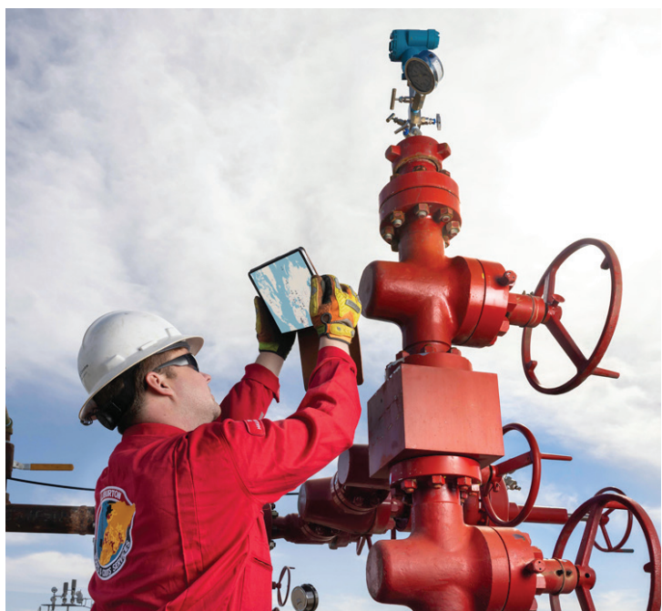
FIG. 3. Close-up inspection of wellhead equipment in the course of a Boots & Coots well control audit.
