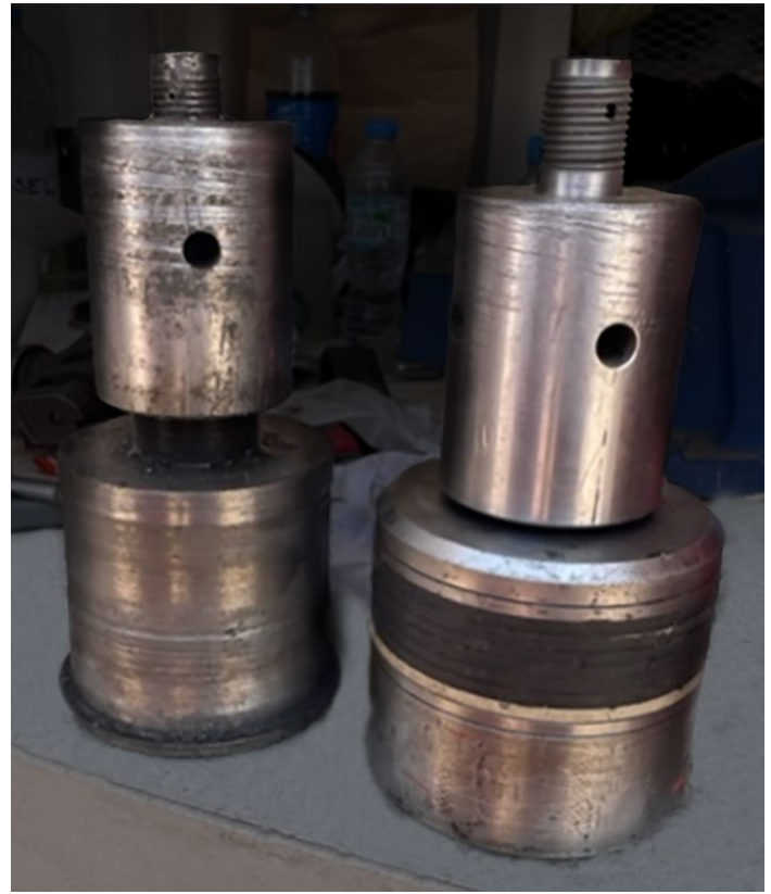
Original plug (right) and after milling and retrieval (left)
