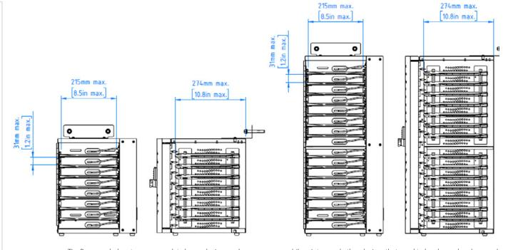
Tip: Remove shelves to accommodate larger devices such as scanners, mobile printers and other devices that need to be charged and secured.
