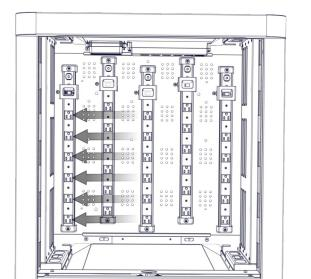
Run the cable up through the hole at the end Pull the cable through the rubber grip.
