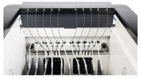
Push the excess cable down behind the cable management bracket and ensure enough cable is pulled through the bracket (depending on device).
