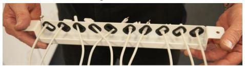
Important: To ensure correct external LED status indication (on the top frame of the Cart), cables should be connected to the correct USB ports on the iQ 5 Sync Charge Boxes (see image below).
