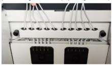
Fit the cable management bracket back into the correct position and replace and tighten the knobs to secure the bracket.
