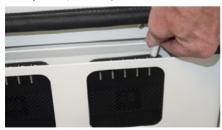
After undoing the two knobs, remove the cable management bracket from the iQ 20 Cart.
