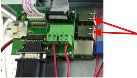
4. Connect your laptop or computer to the FUYL Tower over Ethernet cable. If your FUYL Tower is part of a Local Area Network, it may already be plugged into a wall socket. If not, open the middle control panel with the large key provided, and connect an Ethernet cable from the controller unit's Ethernet socket to your computer.
