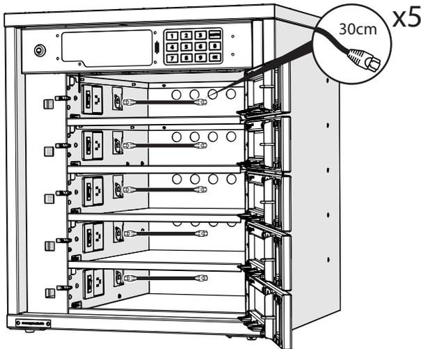
Plug the 30cm ethernet cables to the RJ45 port inside each shelf.
