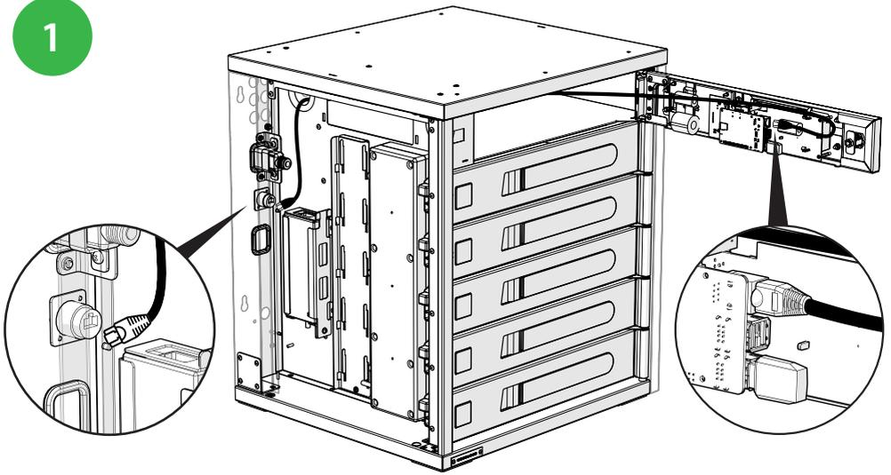
Disconnect the pre-installed ethernet cable from the internal RJ45 port at the rear of the FUYL Tower only.
