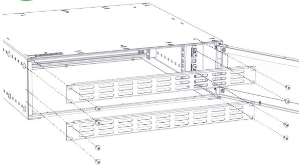
Remove front cover plates and install Network Switch (not included).
