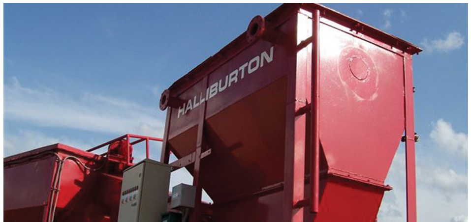
The mobile vertical cuttings dryer is used to treat contaminated cuttings.
