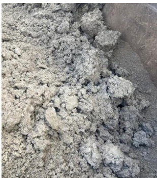
Left: Dried cuttings after processing with vertical cuttings dryer (above).
