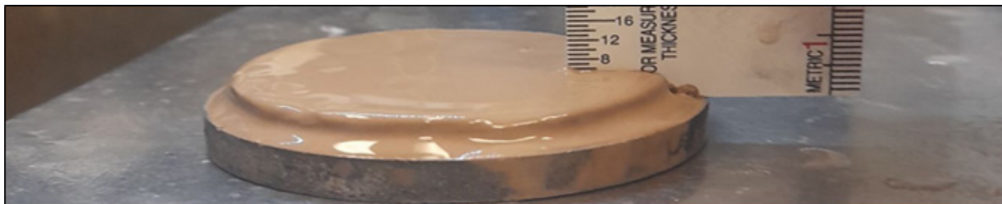
Figure 3: Field fluid: 4,500 psi on 10 µm ceramic disc, 17.2 ppg. Fluid loss = 14.6 ml (total).
