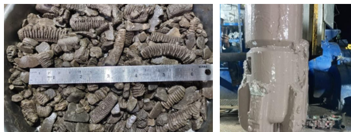
Left: Shale cuttings preserved well enough to exhibit drill bit markings from downhole. Right: Bottom hole assembly with minimal accretion of clays. This is a result of proper inhibition from drilling fluid.
