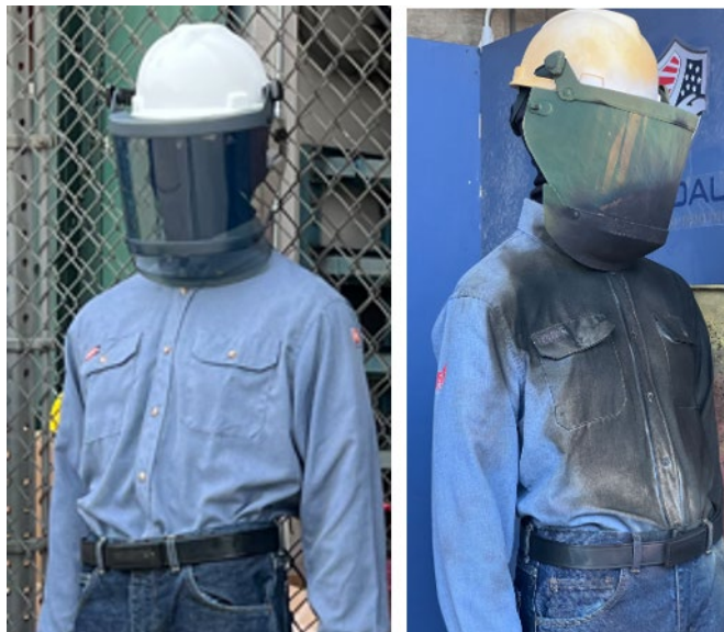
Fig 3. Example Arc-Rated daily wear before and after exposure to DC Arc Flash
