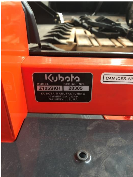
Image 2 : The model and serial numbers can be found on the data plate located on the side of the unit.
