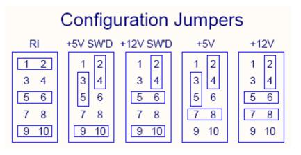
In the switched configuration, power is turned on when the port is opened, and turned off when the port is closed.
