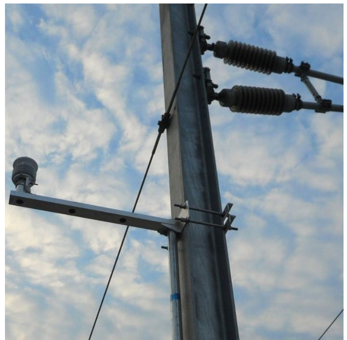
Lufft ultrasonic wind sensor on a railway monitoring system for high-speed trains in China. Credit: OTT HydroMet
