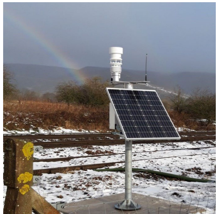
Monitoring station with a compact weather sensor Lufft WS601 (tipping bucket rain gauge). Image: OTT HydroMet
