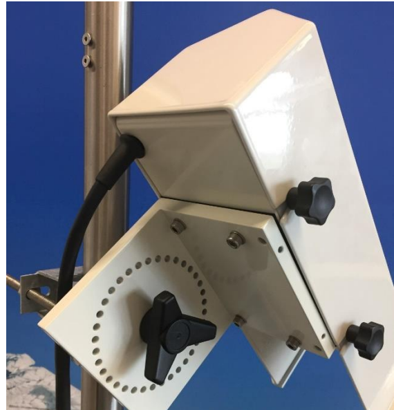
Figure 14: Sensor assembled with hood. After attaching the cable, the weatherproof protective hood is fixed again using the three knurled screws.
