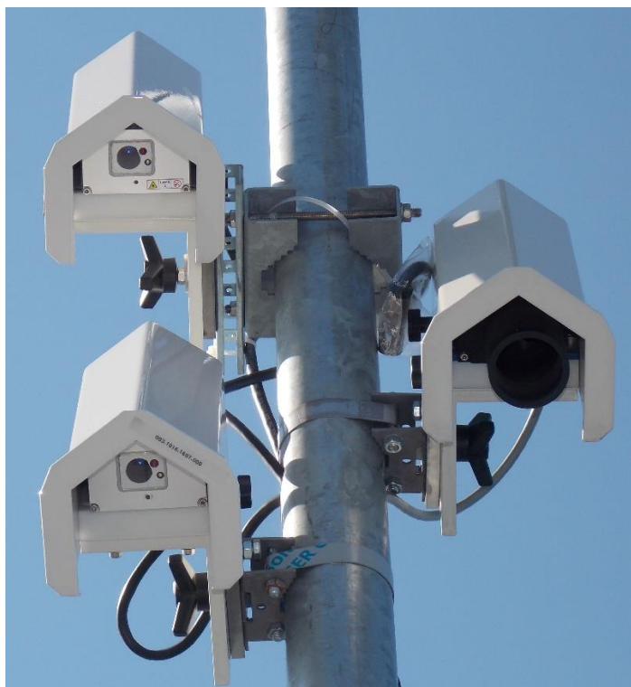
Figure 12: SHM 31 sensors with mast clamp 8365.610-11 (top left), mast clamp 8365.608-11 (bottom left) and SHM 30 sensor with mast clamp 8365.608-11 (middle right).
