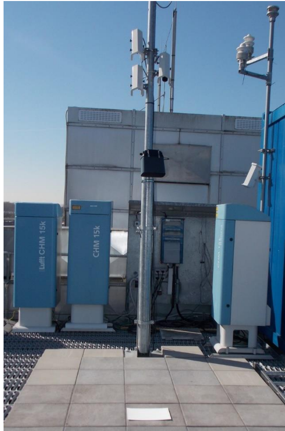
Figure 31: Checking the signal quality with the white card 8365.KWK-WS
