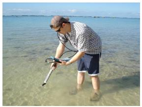
Figure 3. Real-time in vivo phytoplankton measurement using fluorescence sensors on a HYDROLAB sonde
