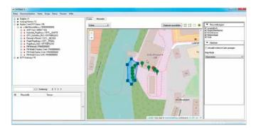
At any time, the user interface map view provides a good overview over the entire measurement network and the status of the individual stations.
