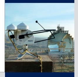
Automatic sun tracker SOLYS2 with a pyrheliometer and two ventilated pyranometers. The ventilation units help to keep the pyranometer domes clean from dust and dew.
