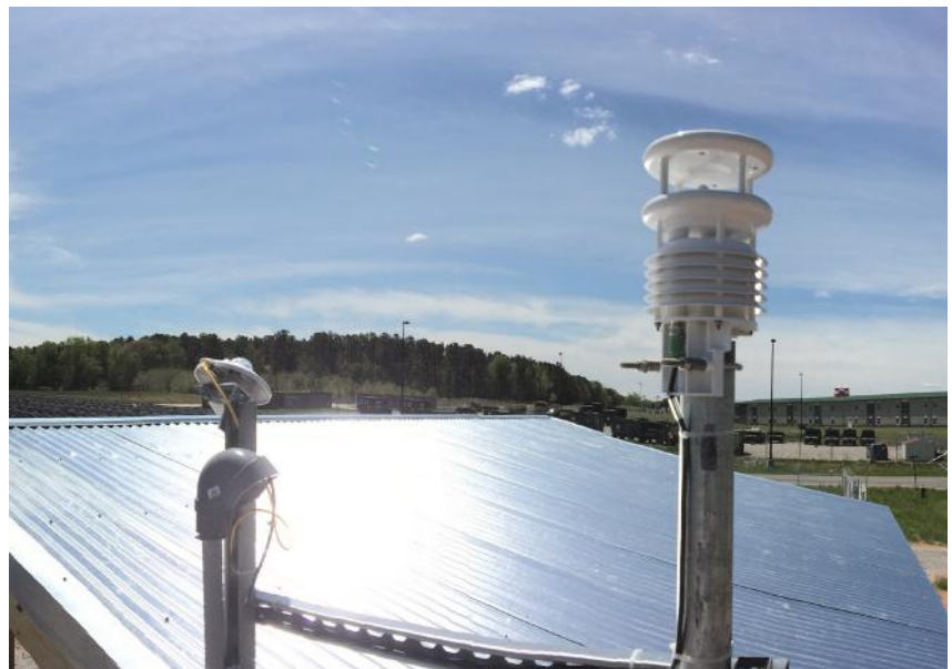
Lufft WS500 weather sensor in the foreground with the installation array behind
