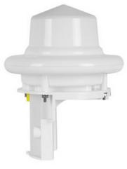
Radar reflection method to measure velocity on hydrometeors by 24-GHz-Doppler radar.
