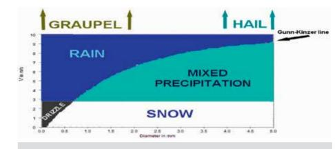
Classification of precipitation by drop size and velocity. The Gunn-Kinzer line indicates the terminal fall velocity for raindrops of various sizes
