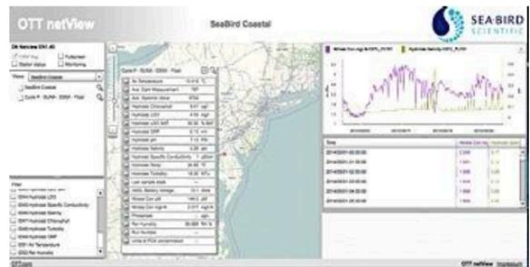
**Figure 3.** Real-time data is collected by an OTT netDL 500 controller and transmitted hourly via the built-in GPRS modem. Data is available online via the OTT netView application.
