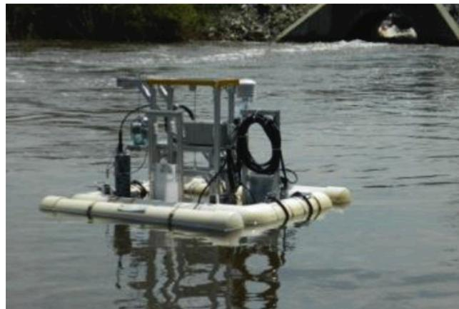
**Figure 1.** Sea-Bird Coastal / Hach Hydromet Foreman Branch Nutrient and Water Quality monitoring platform located on Chino Farms.
