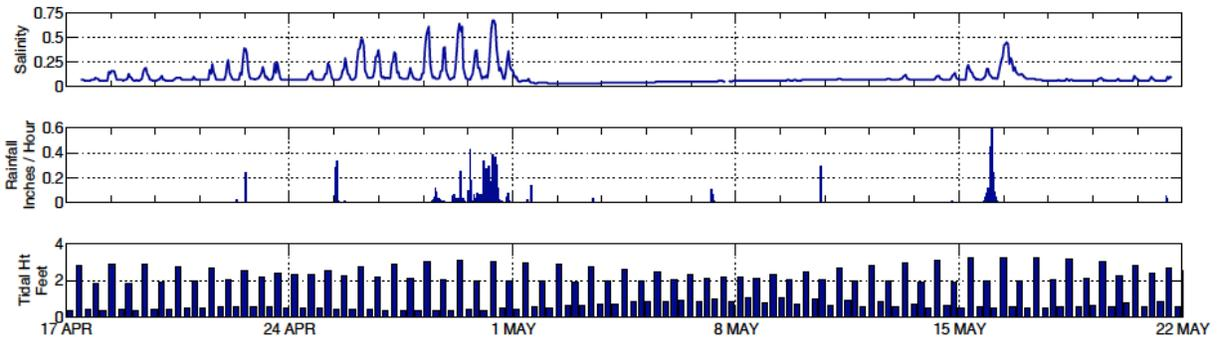
**Figure 4.** The Salinity sensor on the Hach Hydromet D55 clearly resolves the small tidally driven salinity differences between Foreman Branch and the Chester River, until the large rain events in late April and mid May reduce the River salinity to nearly zero.
