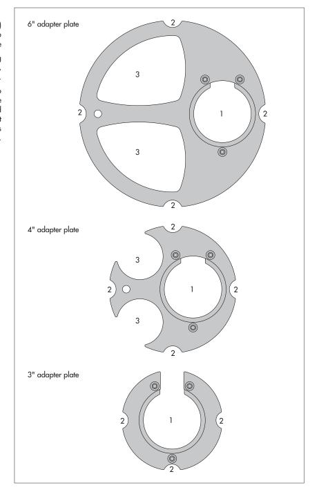
Fig. 7: Accessories for installation – Part 2 1 = drilled hole for OTT ecoLog 800 (3G)
