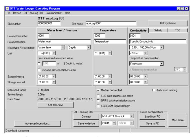
Fig. 16: Setting the OTT ecoLog 800 (3G) operating parameters using the OTT Water Logger Operating Program.
