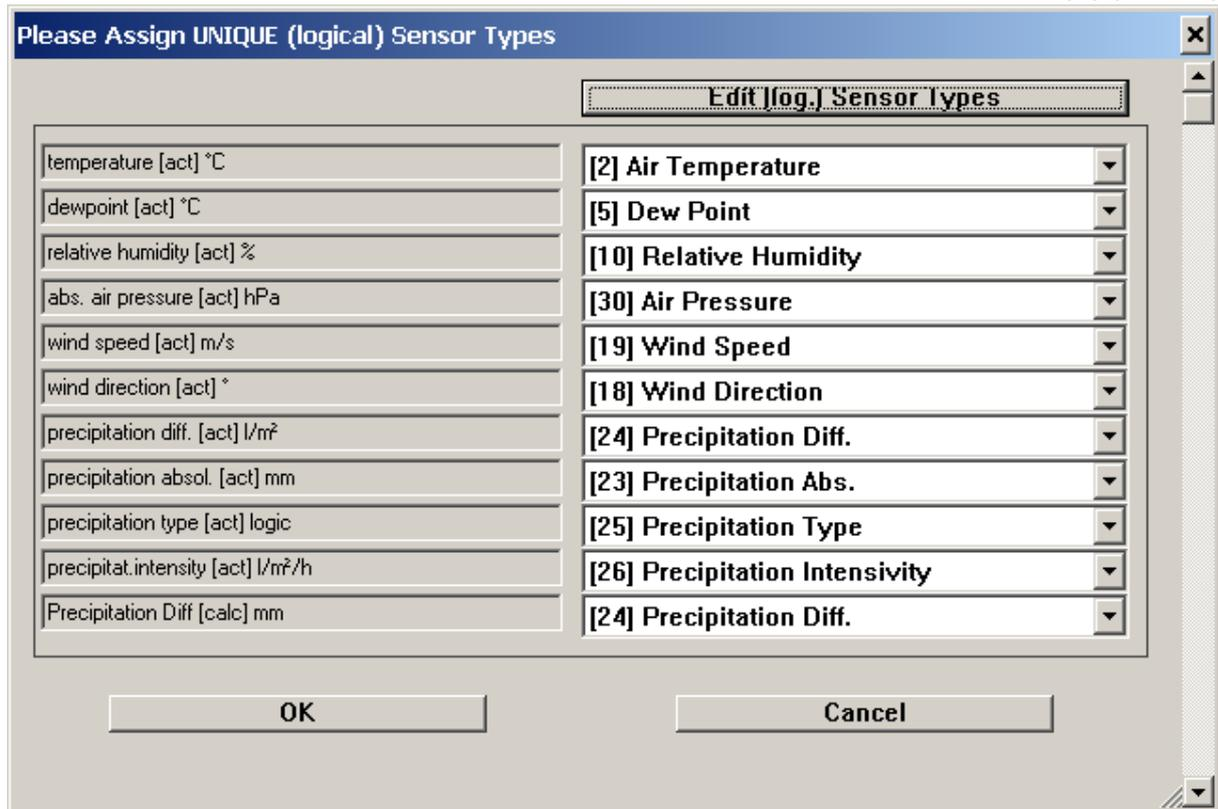
You can select a logical sensor type from the drop down box. If there is no pre-defined sensor type that fits your sensor, you can create a new sensor type using the button "Edit (log.) Sensor Types".
