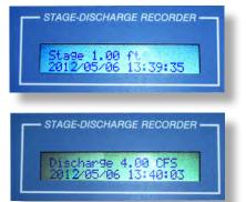
**NOTE:** Software supports only 2 total measurements: Stage & Additional Sensor. Other channels are for future use.
