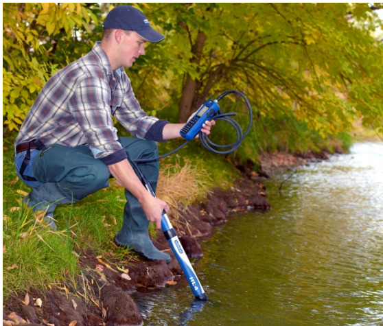
HYDROLAB HL4 multiparamter water quality sonde
