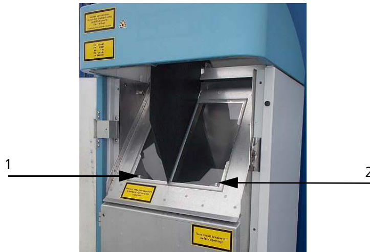
Fig. 28: Glass panels have to be cleaned. In the lower right corner of the receiver window pane the red „error“ light is located.
