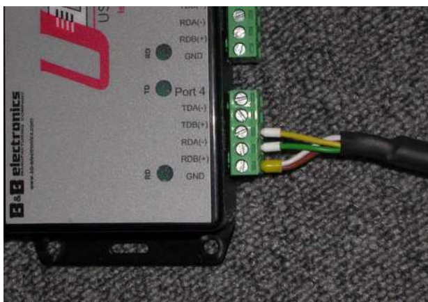
Fig. 10: Connection data cable RS485 (4 wire). Designations RDA(-), RDB(+) are used in different ways by RS485 interface suppliers. Lufft is using the notation from B&B in this manual.
