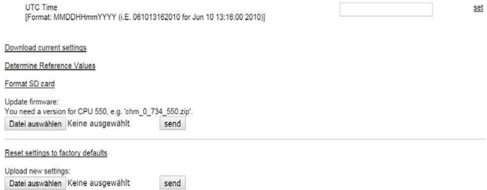
Fig. 20: Web interface, tab config system lower part in service mode: access on system configuration parts. In superuser mode some parameters are not listed for safety reasons.
