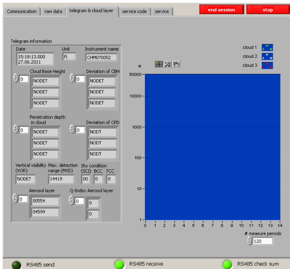
Fig. 34: All types of telegrams contain cloud layer and associated penetration depths; in the advanced and raw data telegrams also the standard deviations of these values and aerosol layers are transmitted. These values are displayed on the left side. The right side shows the course of cloud heights over the last 120 (tbd) telegrams.
