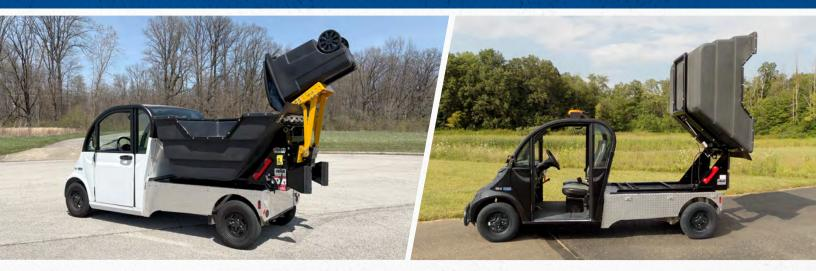
Stellar's Refuse Hopper offers a compact yet powerful solution for waste collection in areas where traditional garbage trucks cannot reach. Designed for efficiency, this eco-friendly system simplifies trash disposal while providing easy maneuverability in tight spaces. With a 2-cubic-yard poly hopper and a hydraulic dump system, it makes waste management faster and more effective in a wide range of applications.
