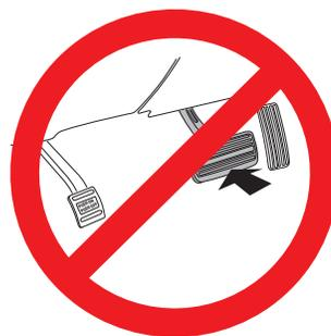
Make sure the body is lining up with the rear rollers while loading. Refrain from using the brake during initial loading of a body. Likewise, do not engage the transmission to use the drivetrain to assist the hydraulics during the loading process.
