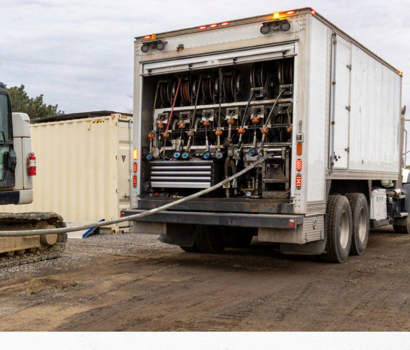
Stellar's comprehensive lineup of fuel and lube trucks and other mobile service equipment — formerly offered under the Elliott Machine Works name — allows you to perform refueling, lube services and preventive maintenance directly onsite, minimizing costly downtime. With customizable configurations and various sizes, these trucks enhance productivity whether you operate a few pieces of equipment or a large fleet.
