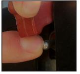
Manual Winch Down: Push the manual winch switch down to lower the cable and hook.
