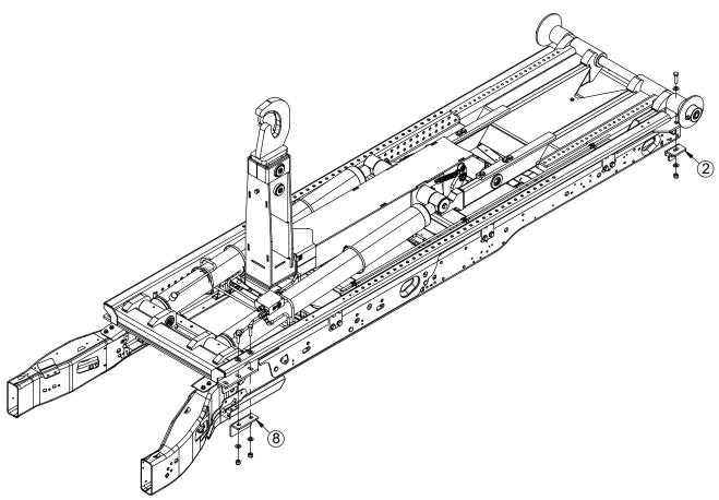
NOTE: BOLT FRONT AND REAR TIE-DOWN ANGLES TO THE UNDERSIDE OF EACH MOUNTING PLATE LOCATED ON THE OUTSIDE OF THE MAIN RAILS OF THE BASE. (BOTH SIDES)
