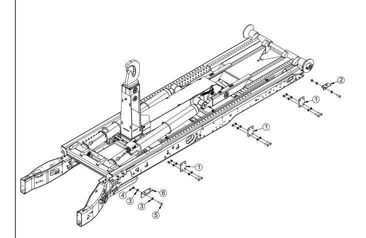
NOTE: BOLT EACH TIE-DOWN ANGLE AND PLATE TO THE TRUCK FRAME (BOTH SIDES).
