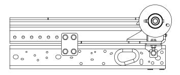
NOTE: MODIFY THE TRUCK FRAME AS NECESSARY SO THAT IT ENDS FLUSH WITH THE REAR TO MOUNT BUMPER.
