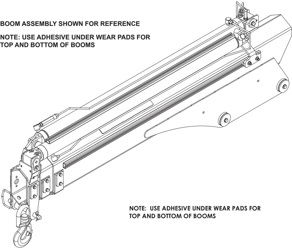
**NOTE: USE ADHESIVE UNDER WEAR PADS FOR TOP AND BOTTOM OF BOOMS**
