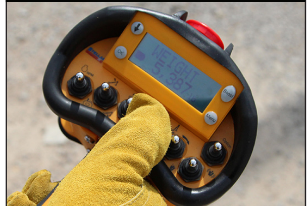
Winch Up/Down Toggle - Load Weight
